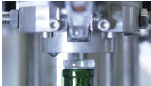
GAI Adapterli yarı otomatik kapama www.youtube.com/watch?v=zNWeQ87UzFE&t=8s
